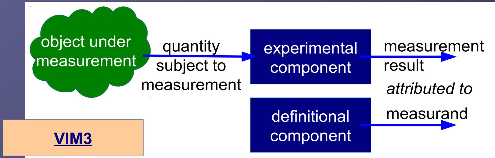
The idea: we do our best to let the measuring system interact with the quantity we want to measure, but the measurement result will be attributed to the quantity as we have defined it, not to the (unknown) quantity with which the instrument actually interacted
